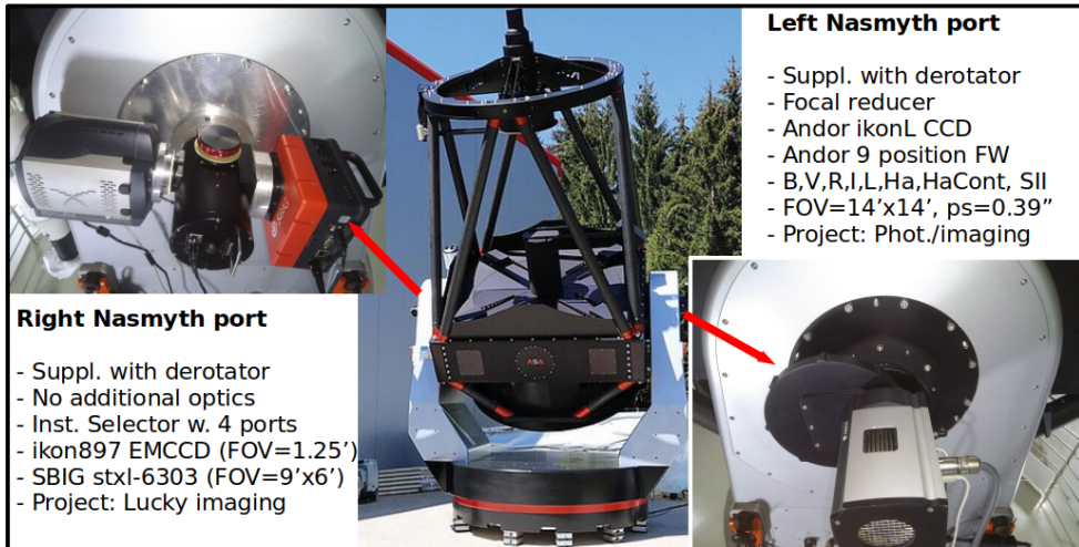
Figure 1: The 1.4m telescope (middle) and the two ports with image-derotator.
